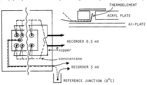
Thermoelements with very small tips are soldered from 2 x 0.1 mm copper-constantane double wire. Ten (or even more) of them are connected in parallel, and two such groups are connected oppositely parallel via a thicker copper cable to a 0.5 mV recording channel. The voltage of this circuit approximates zero in all temperatures. until a fly (or pupa) in contact with one of the thermoelement tips freezes. At
